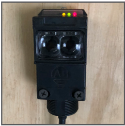
Photo-eye with 10-foot maximum range
